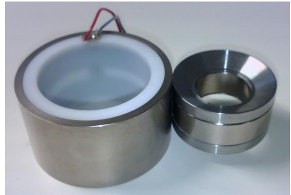
Left: static part consisting of coil and housing Right: moving part on which driving force acts on
